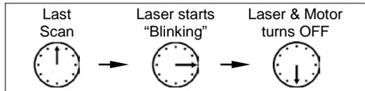
Any movement detected by the IR will “wake” the scanner from the power save mode (see Figure 28).
