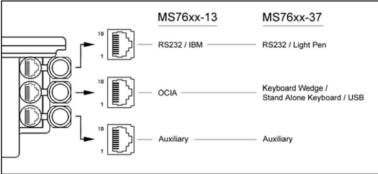
**Figure 22: Connector Orientation**
