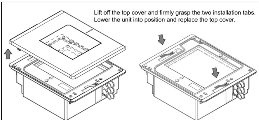
**Figure 9:** Installation Tabs
