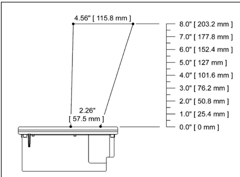
**Figure 30:** Scan Volume in Plane Parallel to Flow
