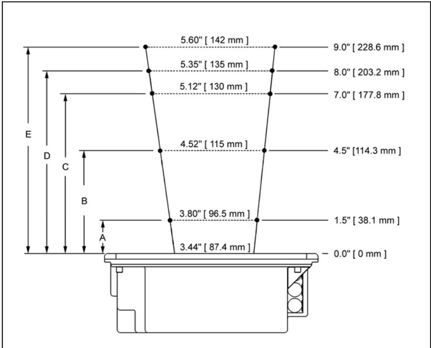
**Figure 31:** Depth of Field Perpendicular to Flow
