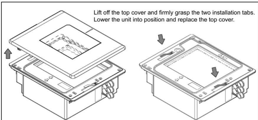
Figure 12: Installation Tabs
