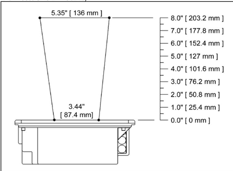
**Figure 29:** Scan Volume in Plane Perpendicular to Flow
