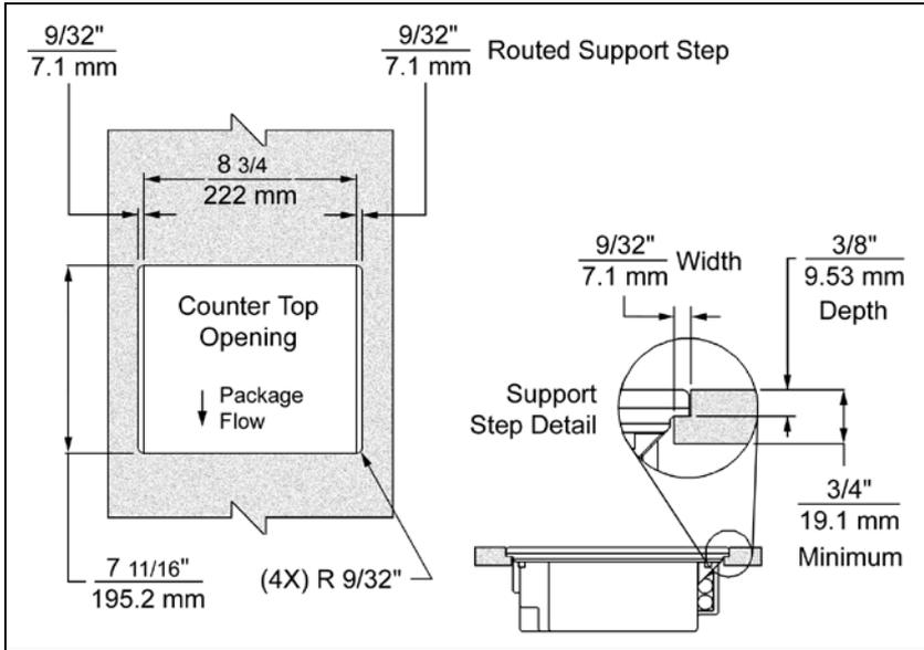
Figure 11: Specifications for Free Hanging Support
