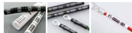
Direct printing on commercially available Soft PVC tubes (inner diameter: 2.5 to 6.5 mm) is possible. Heat Shrinkable tubes Φ3.0 to 6.4mm, Flat tube type materials are also acceptable.\*
