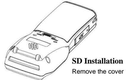
**Figure 3-2** *Installing SD Card*
