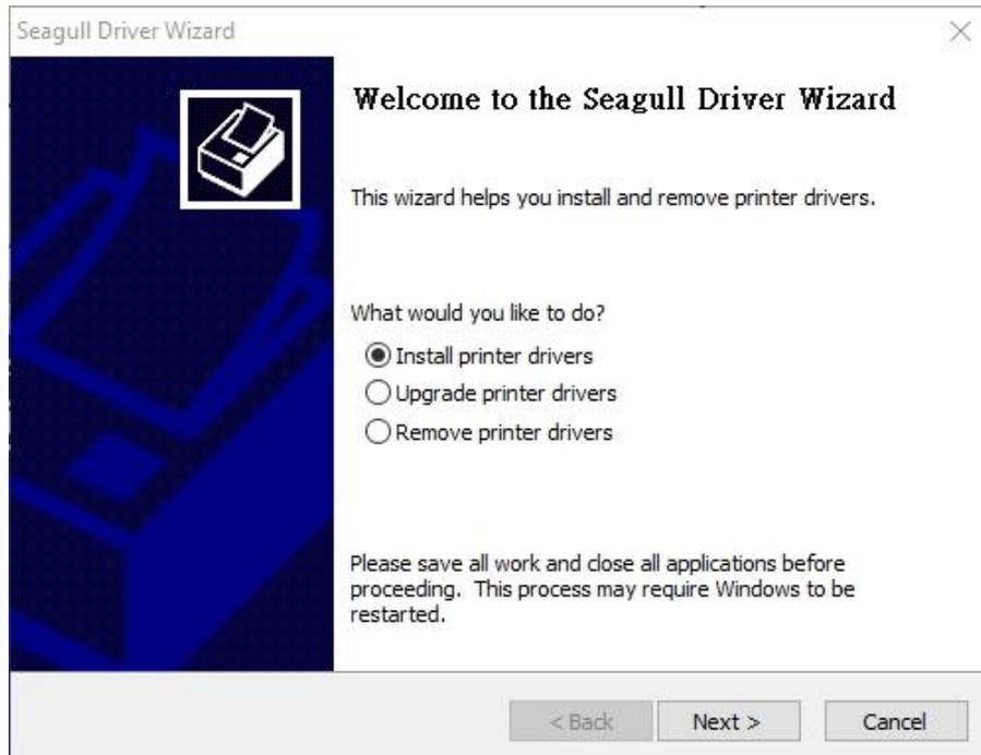
6. On the Seagull Driver Wizard prompt, select the first radio button to "Install a driver for a Plug and Play printer" Then click "Next."
