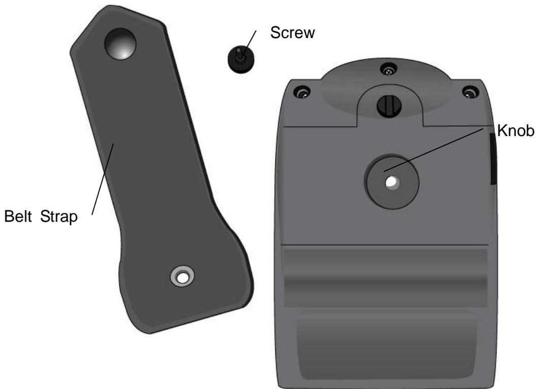
2. Attach the Belt Strap onto the Knob.
